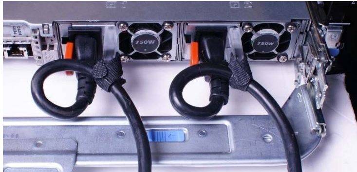
Figure 2. Routing power cables through the strain reliefs
