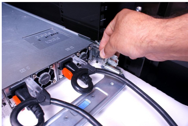
Figure 3. Attaching the inner CMA attachment bracket
