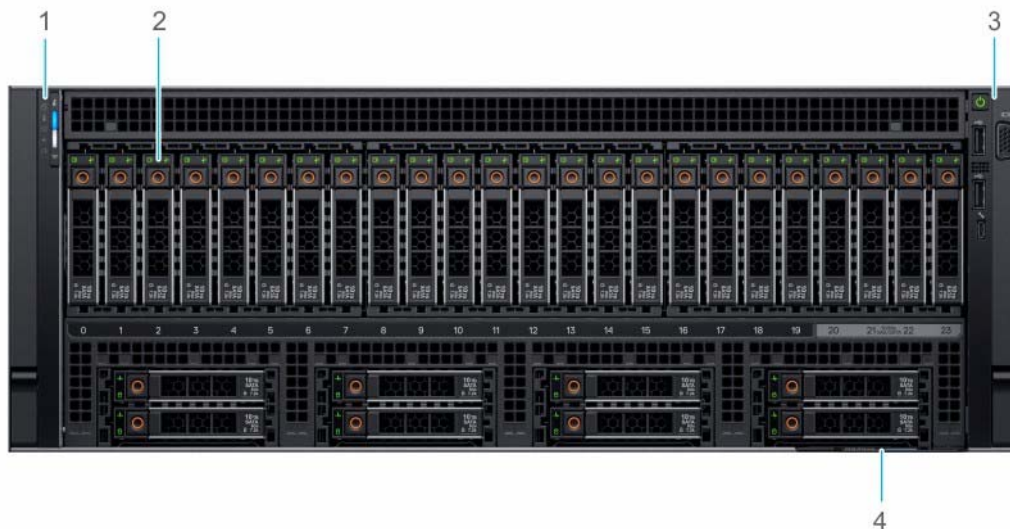
Figure 1. Front view of 32 x 2.5-inch drive system
