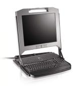
Dell's commitment to large enterprise customers includes offering the infrastructure and accessories that companies need to complement their server installation. The 1U keyboard, monitor, and mouse (KMM) rack console offers IT managers the ability to install a single, integrated user console in a slim 1U (1.75") form factor.
