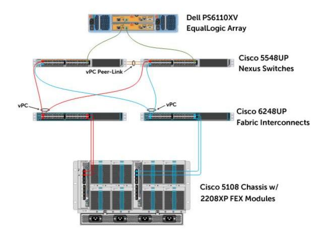
Figure 2. Cisco UCS solution rear view
