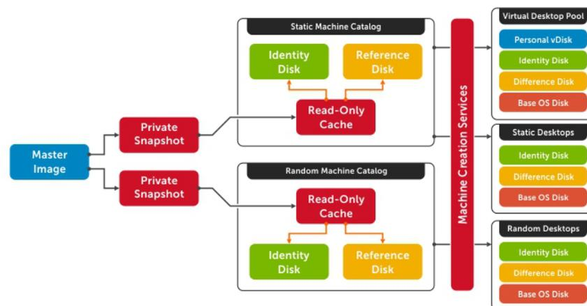
While traditionally used for small to medium sized XenDesktop deployments, MCS can bring along with it some substantial Tier 1 storage cost savings because of the snapshot/identity/difference disk
