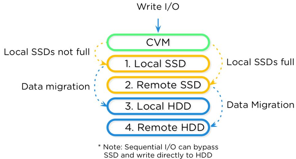
With the DSF, a CVM writes data to local flash memory for fast acknowledgment; the CVM also handles read operations locally for reduced latency and fast data delivery.
