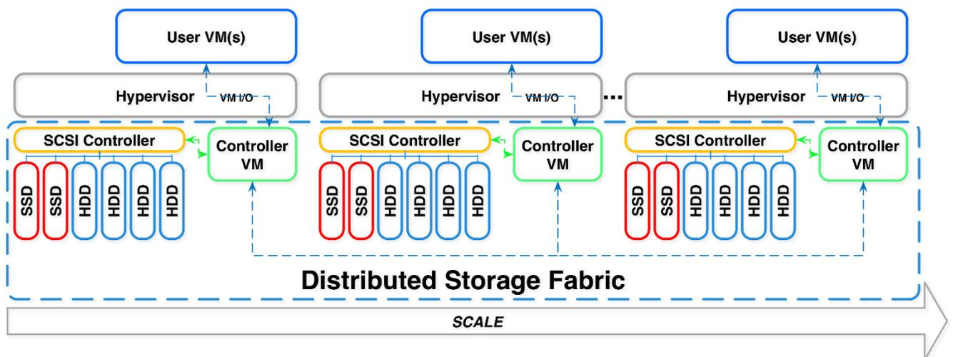
Local storage for each Nutanix node in the architecture appears to the hypervisor as one large pool of shared storage. This allows the DSF to support all key virtualization features. Data localization maintains
