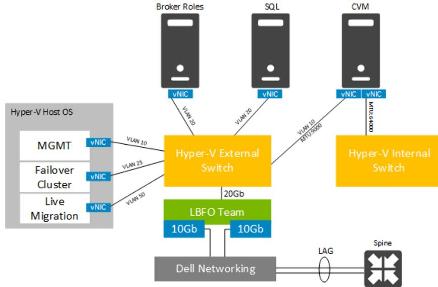
The NIC team for the Hyper-V switch is configured as switch independent, dynamic for the load balancing mode with all adapters set to active. This team is used exclusively by Hyper-V.
