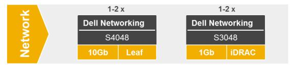
Each Dell EMC S2D Ready Node is equipped with dual port RDMA network adapters for host and storage traffic. Although the solution can function with a single switch, Dell EMC highly recommends redundant top-of-rack S4048 switches. Each RDMA port is connected to a different S4048 switch in this scenario.
