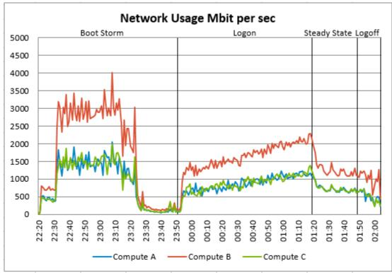
The peak Cluster IOPS for the test run was 6619 IOPS during Logon phase, while the average in Steady State was 1877 IOPS. This data was captured from the sum of the "PhysicalDisk(x)\Disk Transfers/sec" metrics for the mounted virtual disks only. Based on these numbers each user session generated 3.57 IOPS.
