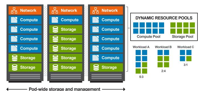
While this paper describes a Dell EMC-enabled OpenStack cloud implementation, Intel<sup>®</sup> Rack Scale Design can also support other cloud frameworks (e.g., Microsoft™ or VMware™) allowing administrators to manage solutions running several clouds from different vendors – all running on the same underlying hardware, and all with the ability to define, allocate and re-allocate resources quickly and independently, as necessary.
