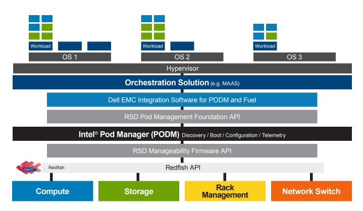
Intel® Pod Manager acts as a resource manager for disaggregated pools of hardware resources by communicating using standard Redfish APIs to hardware-aware software within the DSS 9000 called the Pooled System Management Engine (PSME). PODM provides configuration management of the pools of compute, storage and networking resources to administrators and applications through a vendor-agnostic orchestration (RESTful) API. (See Figure 2).
