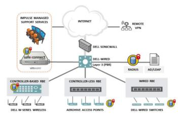
SafeConnect's Network Access Control (NAC) architecture utilizes Layer 3 Policy Based Routing (PBR) and Layer 2 RADIUS-Based Enforcement (RBE) technology to offer the industry's broadest range of device enforcement options.
