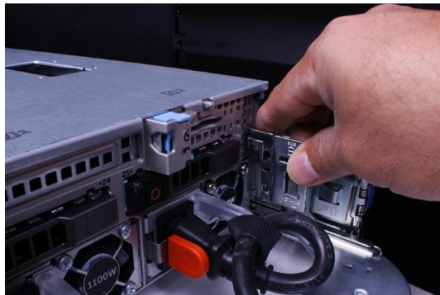
Figure 3. Attaching the inner CMA attachment bracket
