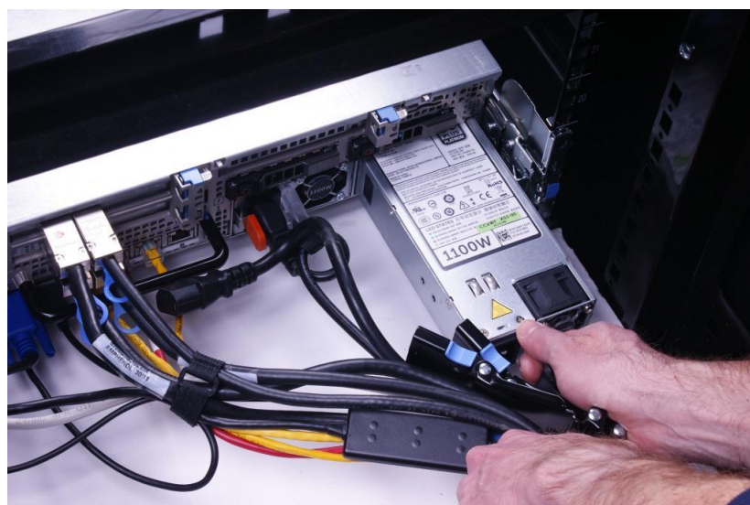
Figure 8. Replacing the outer power supply
