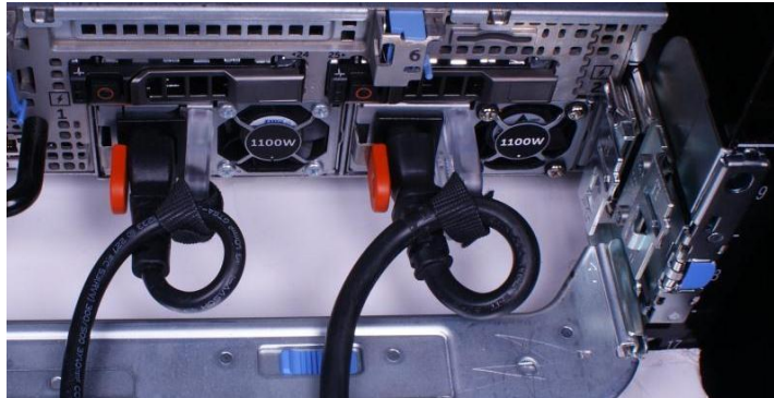
Figure 2. Routing power cables through the strain reliefs
