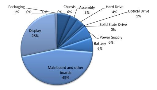
Figure 4: Breakdown of manufacturing phase in the carbon footprint. Total manufacturing contribution is  $253 \text{ kgCO}_2\text{eq}$ , or 68% of the total carbon footprint.
