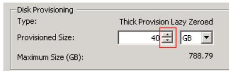
For Windows machines: After growing the virtual disk from the vSphere client, an administrator must log into the virtual machine, rescan for new disks, and then use DISKPART or the disk management MMC console to extend the drive.
