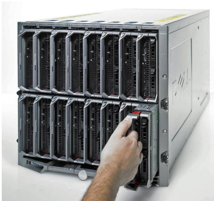
Figure 8 Modular Server Removal
