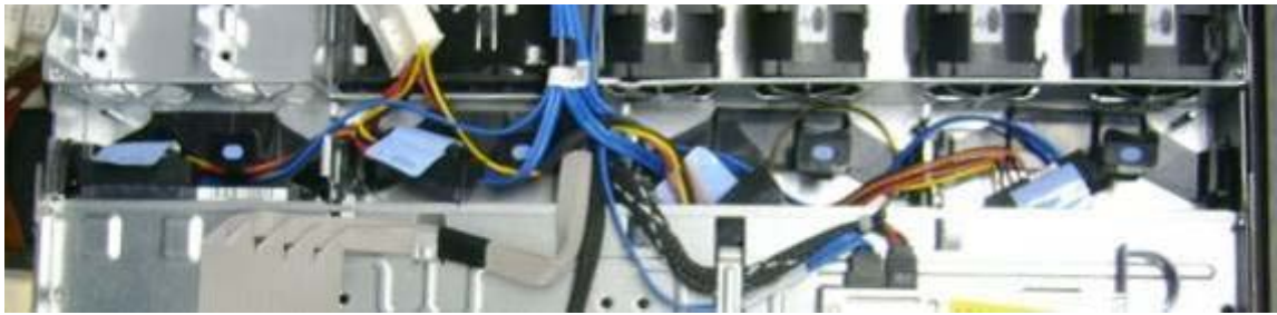
Figure 35. Top-View for Cabled HDD Connection
