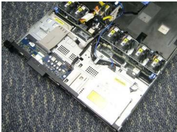
Figure 33. Hot-Swap HDD Configuration with Backplane
