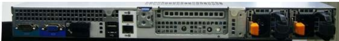
Figure 6. With Redundant Power Supply
