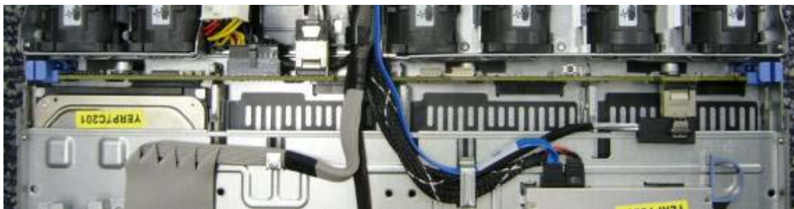
Figure 34. Top-View for Hot-Swap HDD Connection
