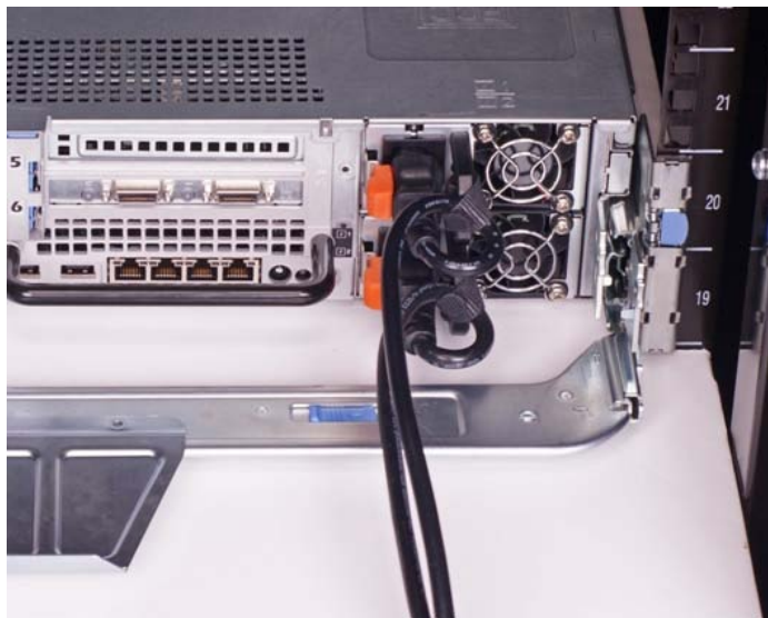
Figure 2: Routing Power Cables Through the Strain Reliefs
