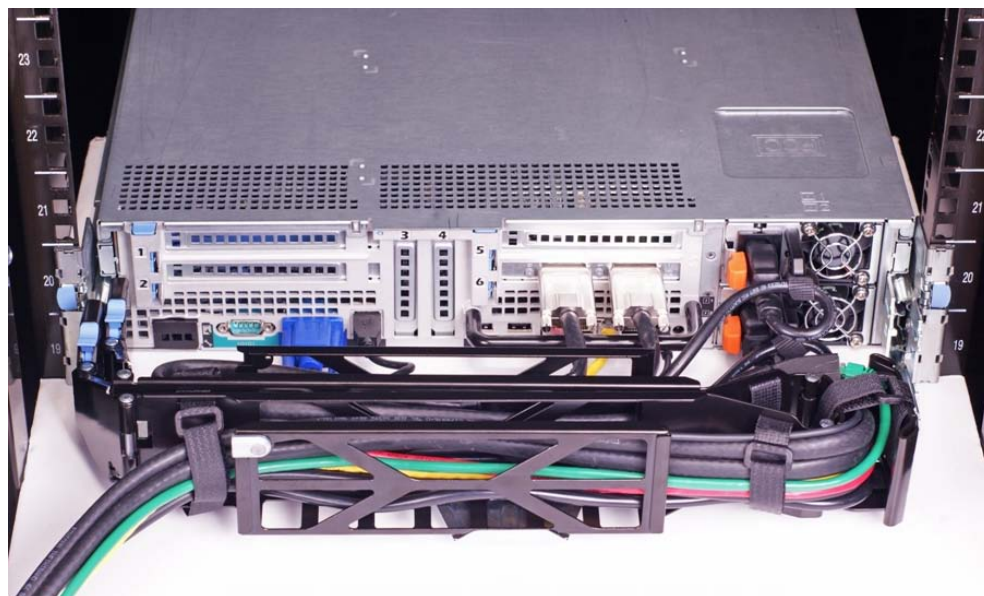
Figure 4: Left-Side Mounted CMA Installation
