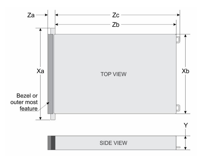
Figure 8. Chassis dimensions
