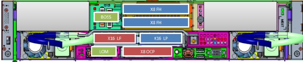
Figure 7. Rear view of the system with riser config 0: direct attach NVMe cards (either 6x NVMe direct attach or 4x NVMe direct attach + 4 Universal slots)
