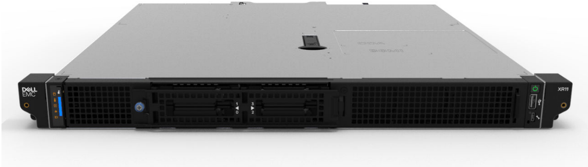
Figure 2. XR11 Rear accessed chassis front view, no bezel
