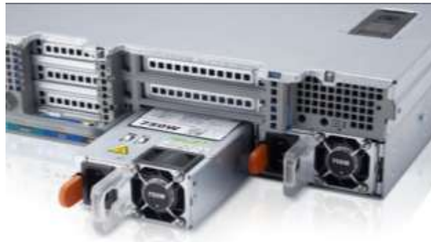
Figure 8. 750W power supply unit
