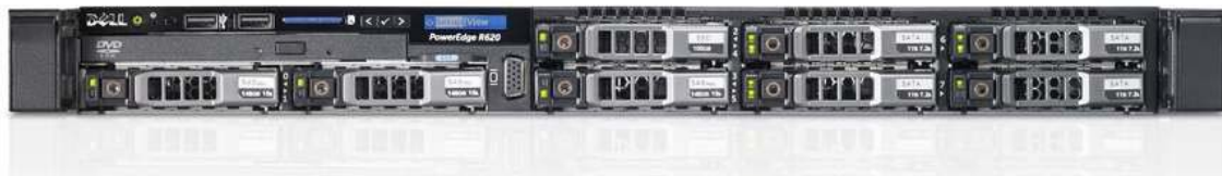
Figure 1. Eight-drive bay chassis front view without bezel
