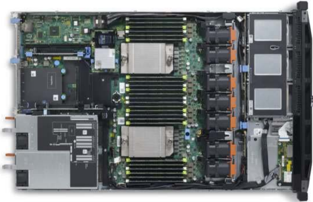
Figure 5. Eight-drive bay chassis internal view
