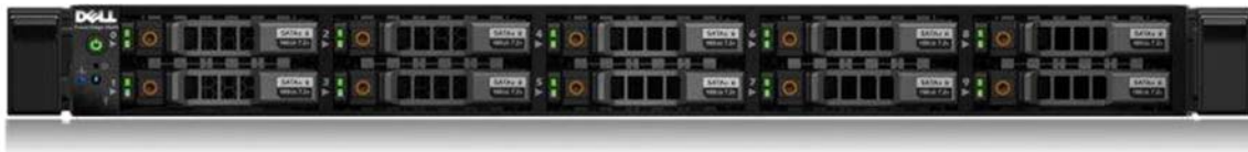
Figure 2. 10-drive bay chassis front view without bezel
