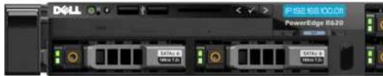
Figure 6. LCD control panel for 8-drive bay chassis
