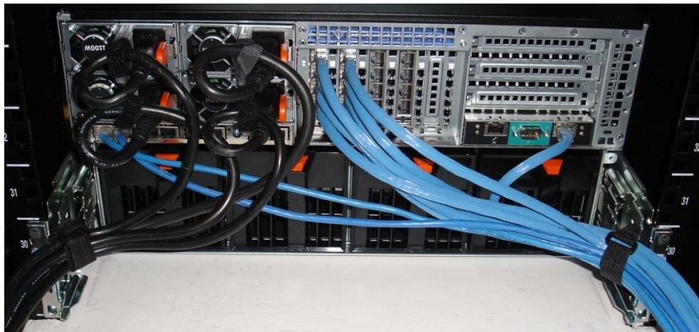
Figure 8. Cable routing without a CMA
