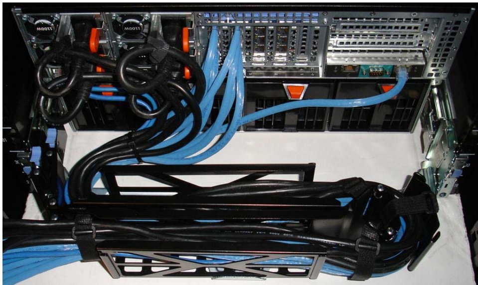
Figure 5. Right-side mounted CMA installation
