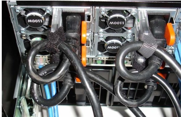
Figure 2. Routing power cables through the strain reliefs
