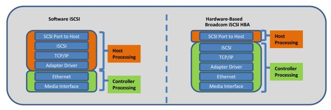
Broadcom's iSCSI offering is based on Broadcom's hardware offload architecture designed to deliver dependable performance, low CPU utilization, reliability, and unified NIC and storage management using the Broadcom Advanced Control Suite (BACS) management application for both 1 GbE and 10 GbE networks. Benefits include:
