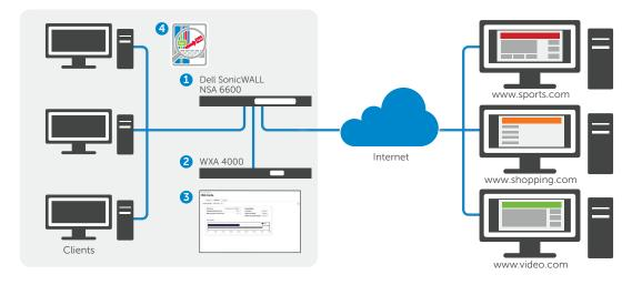
**1** Dell SonicWALL Next-Generation Firewall appliances provides Deep Packet Inspection scanning for malware and intrusions.
