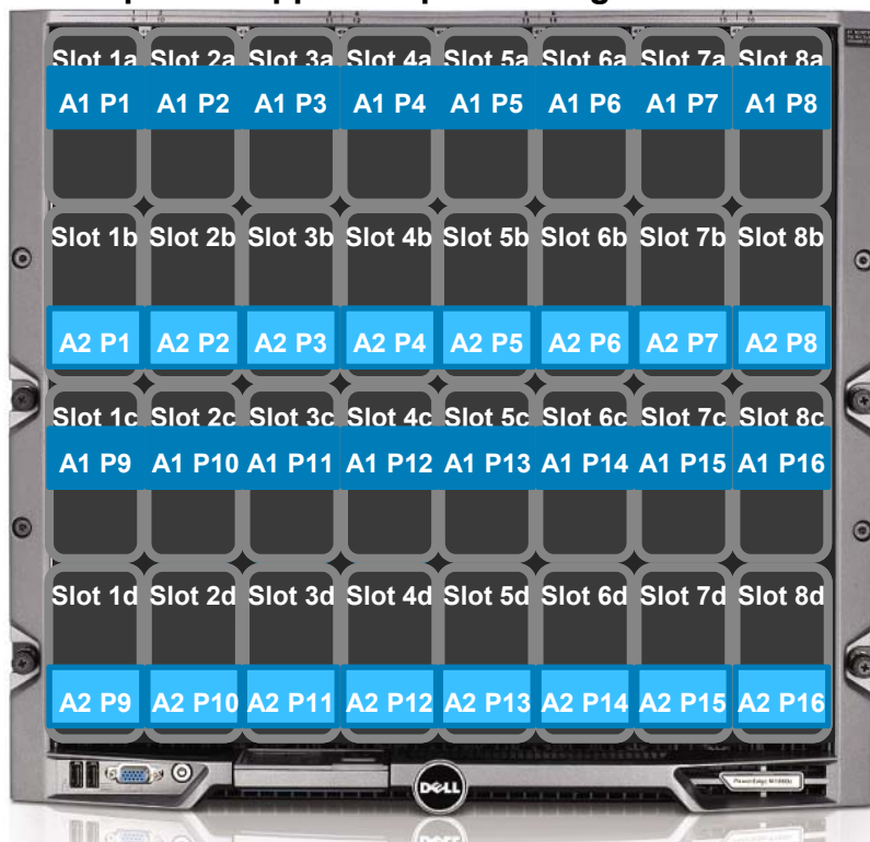
IOM ports mapped to quarter height blade slots
