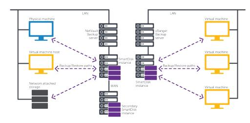
NetVault SmartDisk's ability to share disk-based backup storage across heterogeneous platforms eases administrator workloads by providing a single data protection solution.
