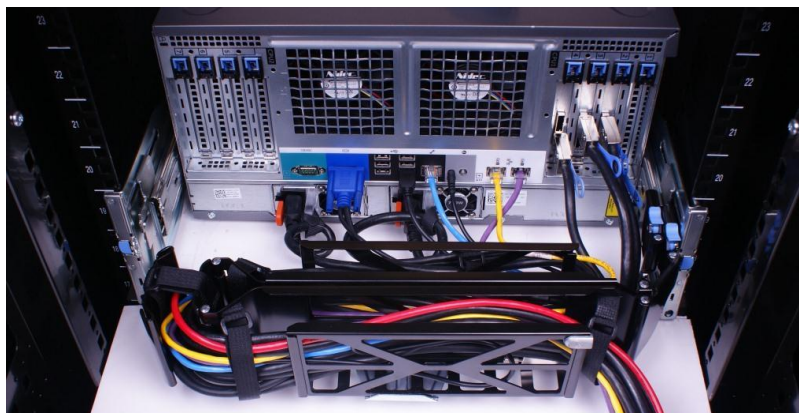
Figure 5. Right-side mounted CMA installation
