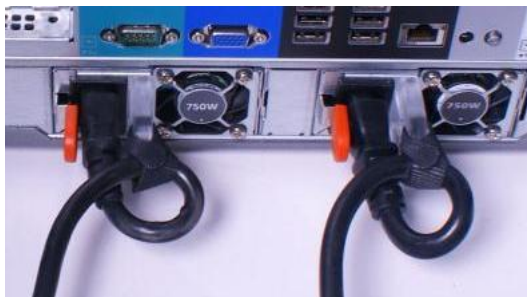
Figure 2. Routing power cables through the strain reliefs
