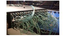
132 x 40GE QSFP+ ports Once connectivity between the Ixia XG12 and the Dell Z9500 was confirmed, we did not have to re-cable for the duration of the testing.
