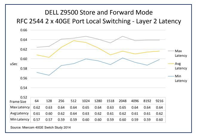
Average latency for the Dell Z9500 in locally switched Layer 2 store and forward mode ranged from only 0.60 to 0.64  $\mu$ sec.
