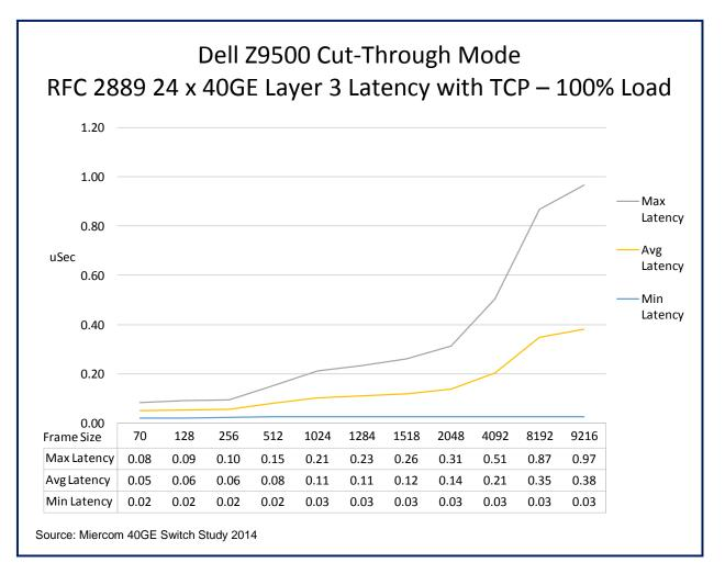
The Dell Z9500 with 24 active ports with fully meshed traffic in cut-through, exhibits consistent low latency up through 2048-byte packets on all connected ports. From the smallest packet size of 70-bytes to the largest 9,216-bytes, the average latency ranges from 0.05 to 0.38  $\mu$ secs. Tests were conducted in accordance with RFC 2889.
