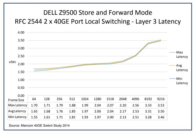
Average latency for the Dell Z9500 x-fabric store and forward mode ranged from 1.65 to 3.50  $\mu$ sec.
