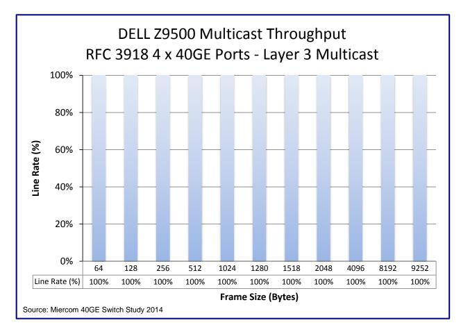
The Dell Z9500 switch exhibited line rate throughput for Layer 3 IPv4 traffic using RFC 3918 standard tests. The Z9500 achieved 100% line rate throughput for Layer 3 IPv4 multicast traffic for all frame sizes from 64 bytes to 9252 bytes. An Ixia XM12 conducted the test on the Z9500.
