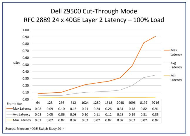
The Dell Z9500 with 24 active ports with fully meshed traffic in cut-through, exhibits consistent low latency up through 2048-byte packets on all connected ports. From the smallest packet size of 64-bytes to the largest 9,216-bytes, the average latency ranges from 0.05 to 0.35  $\mu$ secs. Tests were conducted in accordance with RFC 2889.
