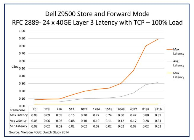
Dell Z9500 with 24 active ports with fully meshed traffic in store and forward mode, exhibits consistent low latency up through 2048-byte packets on all connected ports. From the smallest packet size of 70-bytes to the largest 9,216-bytes, the average latency ranges from 0.05 to 0.31  $\mu$ secs. Tests were conducted in accordance with RFC 2889.
