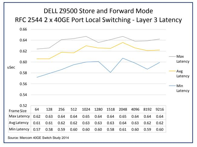
Average latency for the Dell Z9500 in locally switched Layer 3 store and forward mode ranged from only 0.61 to 0.64  $\mu$ sec.
