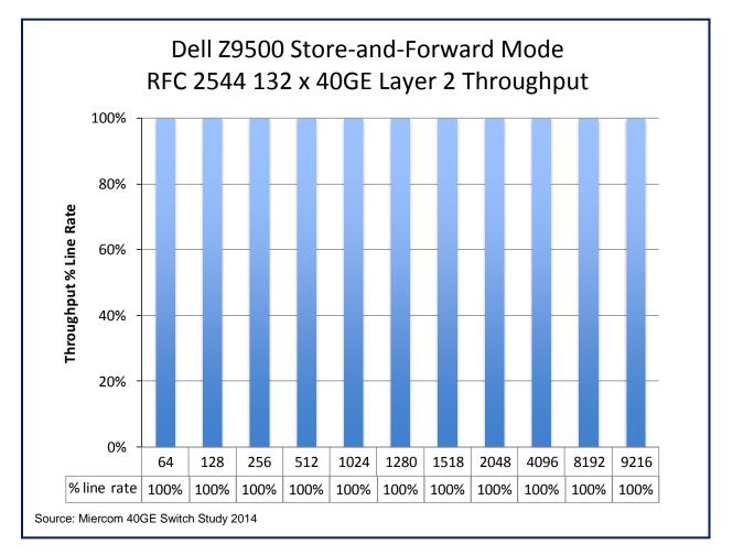
The Dell Z9500 exhibited full line-rate forwarding performance for all packet sizes in this throughput test, conducted in accordance with RFC 2544. No frame loss occurred as the Z9500 operated in store-and-forward mode, with all 132 x 40GE ports fully loaded with Layer 2 traffic.
