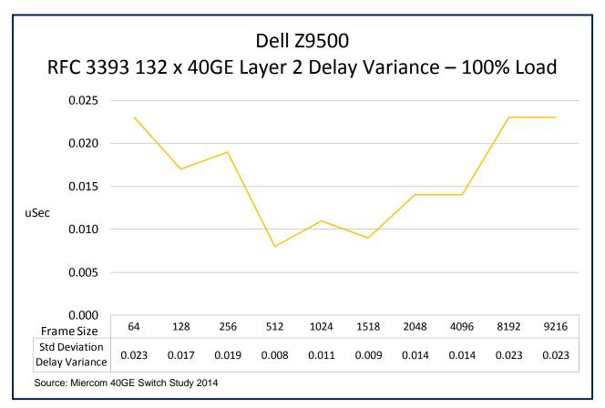
The Dell Z9500 with eleven 12 Port 40G line cards exhibited very little variance in latency - also called "jitter" – less than one quarter of a microsecond on average for all packet sizes up to 9,216 bytes. The Dell switch configured with 132 ports was subjected to a 100 percent traffic load. Layer 3 IP unicast traffic was used for the specified frame size. Tests were conducted in accordance with RFC 3393.
