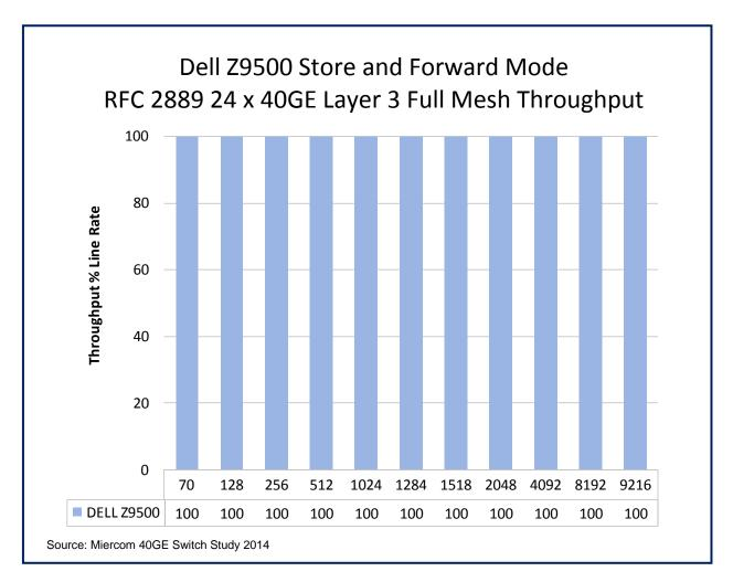
The Dell Z9500 had 12 connected ports each on two separate line cards running full mesh traffic over 24 ports from the Ixia test system. The switch fabric exhibits full line-rate forwarding performance with ports fully loaded without loss for Layer 3 (IP) traffic for all frame sizes. Testing was conducted in accordance with RFC 2889.
