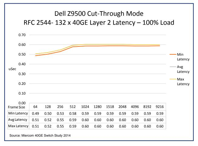
Average latency for the Dell Z9500 in cut-through mode ranged from only 0.51 to 0.60  $\mu$ sec.
