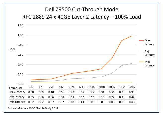
The Dell Z9500 with 24 active ports with fully meshed traffic, exhibits consistent low latency up through 2048-byte packets on all connected ports. From the smallest packet size of 64-bytes to the largest of 9,216-bytes, the average latency ranges from 0.05 to 0.42 microseconds. Tests were conducted in accordance with RFC 2889.
