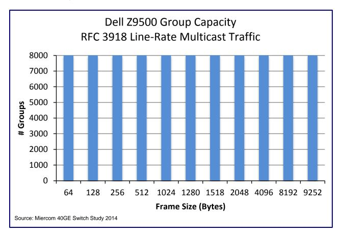
Group capacity was measured by the XM12 by changing the number of multicast groups at a given frame size at line rate multicast traffic to find the maximum number that can sustain 0% packet loss.
