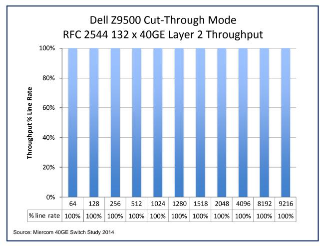
The Dell Z9500 exhibited full line-rate forwarding performance for all packet sizes in this throughput test, which was conducted in accordance with RFC 2544. No frame loss occurred as the Z9500 operated in cut-through mode, with all 132 40GE ports fully loaded with Layer 2 traffic.
