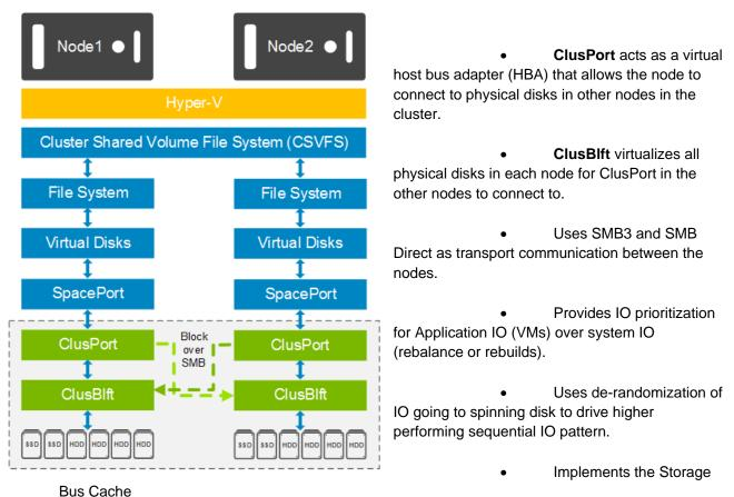
**Storage Bus Layer Cache.** The Software Storage Bus dynamically binds the fastest drives present (e.g. SSD) to slower drives (e.g. HDDs) to provide server-side read/write caching that accelerates IO and boosts throughput.
