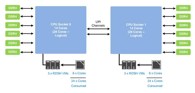
**NOTE:** To ensure no NUMA spanning, remove the checkmark for "Allow virtual machines to span physical NUMA nodes" in the Hyper-V settings of the compute host(s). Also ensure "Maximum NUMA nodes allowed on a socket" is set to a value of 1. This setting is found under Processor > NUMA for each RDSH VM.
