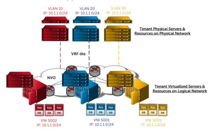
Figure 2 VRF-lite used in conjunction with VXLAN Network Overlay in a virtualized environment
