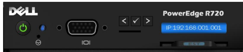
Figure 9. R720 LCD control panel
