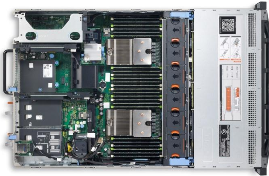
Figure 8. R720xd internal chassis view
