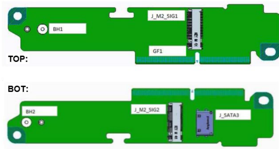
Figure 8. M.2 X 16 SATA Riser PCB Dimension
