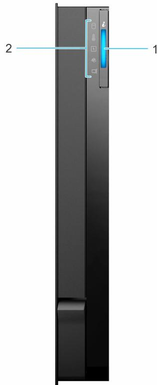
Figure 2. Left control panel
