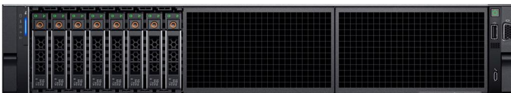
Figure 3. Front view of 8 x 2.5-inch drive system
