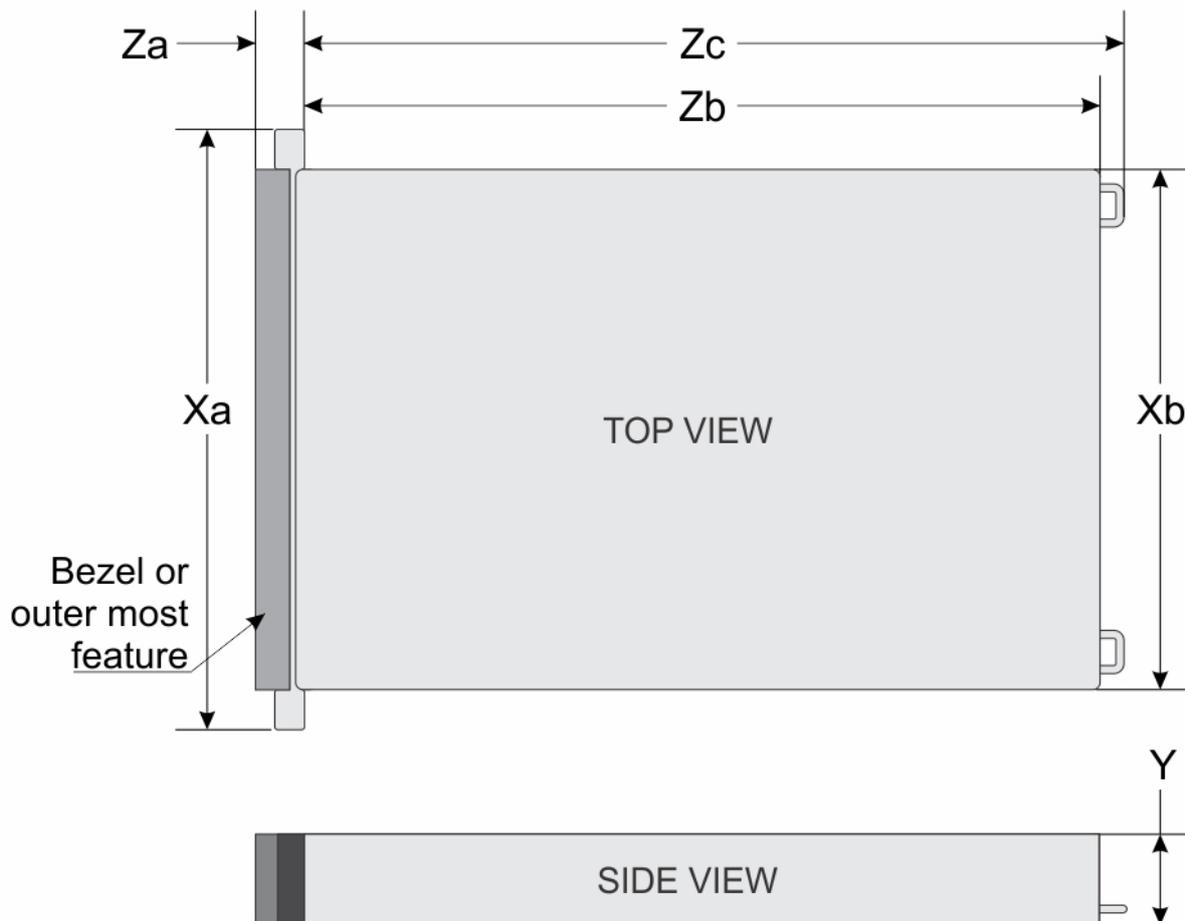
Figure 55. Chassis dimensions
