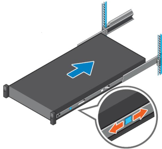
Figure 43. Slide system into the rack
