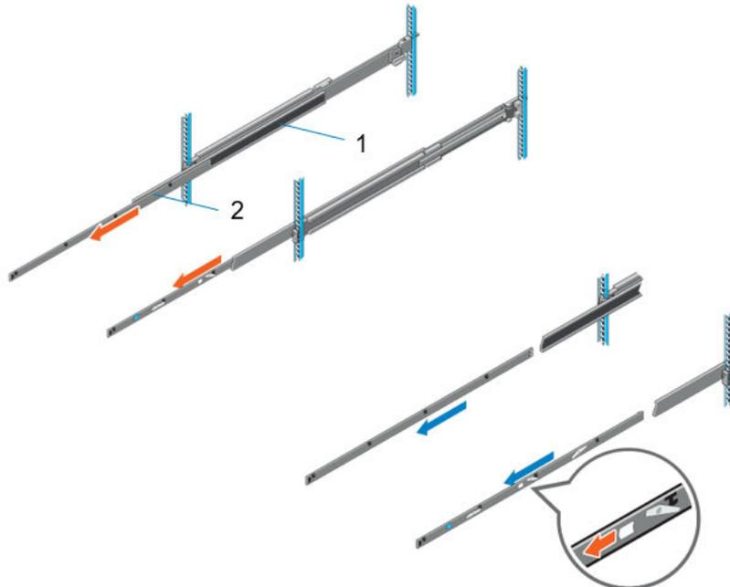
Figure 44. Pull out the intermediate rail
