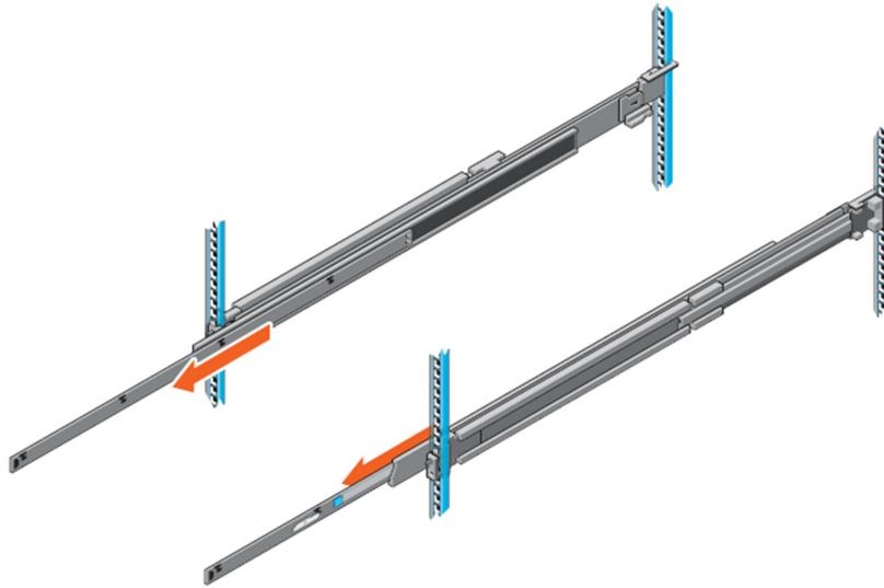
**Figure 41. Pull out inner rail**
