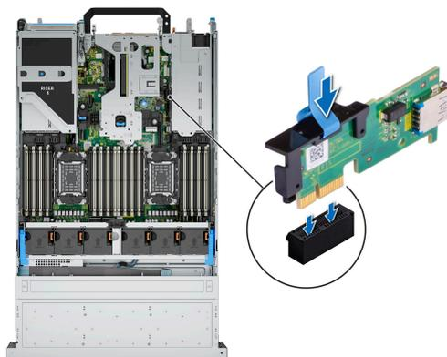
Figure 58. Internal USB Port
