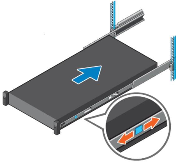
Figure 47. Slide system into the rack
