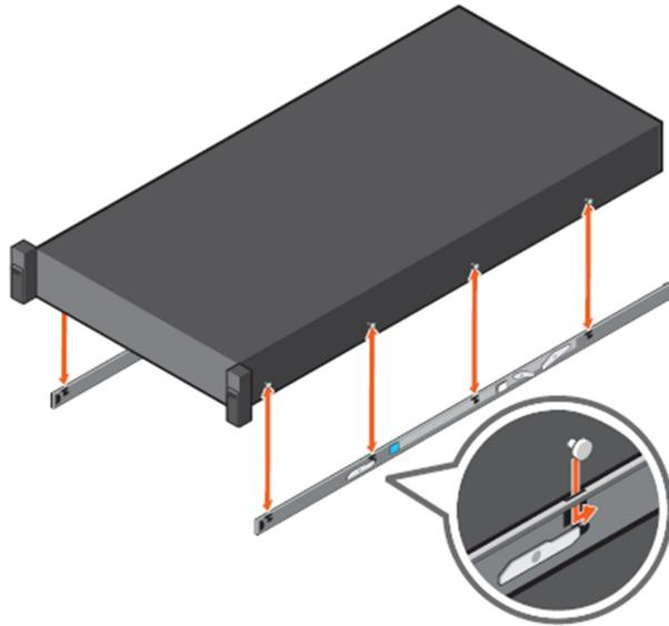
**Figure 45. Attach the inner rails to the system**
