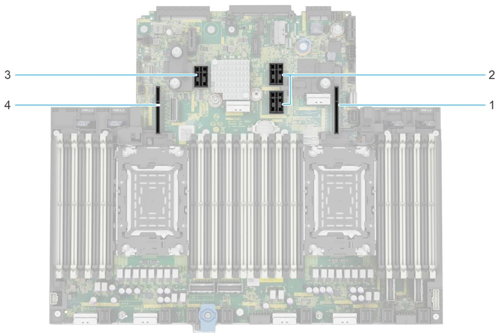
**Figure 13. Riser connector location on system board**
