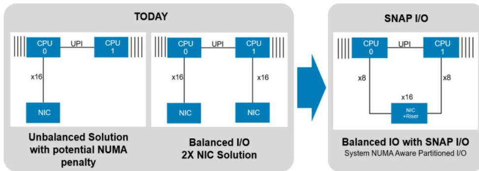
**Figure 15. Comparing an unbalanced one-NIC solution and a balanced two-NIC solution to a SNAP I/O one-NIC solution.**
