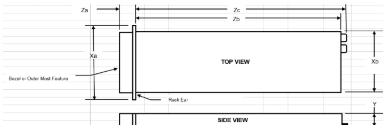
Figure 36. Chassis dimensions
