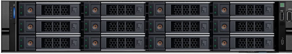
Figure 4. Front view of 12 x 3.5-inch drive system
