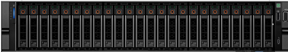
Figure 1. Front view of 24 x 2.5-inch drive system
