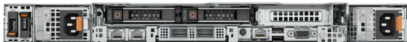
Figure 4. Rear view of the R660 with 2x 2.5 inches Storage drives, 1x LP
