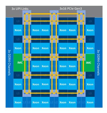
In the Intel<sup>®</sup> Xeon<sup>®</sup> Scalable processor platform Intel<sup>®</sup> Mesh Architecture with up to 28 cores (per processor), the Last Level Cache (LLC), six memory channels, and 48 PCIe<sup>\*</sup> channels are shared among all the cores, giving access to large resources across the entire die and creating dynamic scalability without sacrificing performance.
