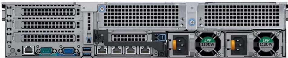
R740 Rear view - with 4x PCIe slots available with riser 2 and riser 3 blanks
