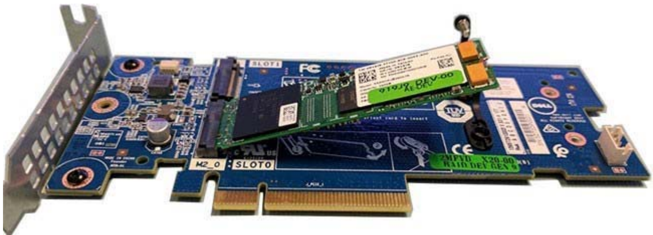
Figure 13. Boot Optimized Storage Subsystem (BOSS)
