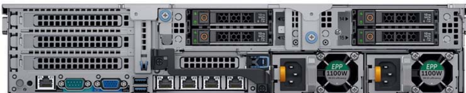
R740xd Rear view - with 4 x 2.5" backplane installed
