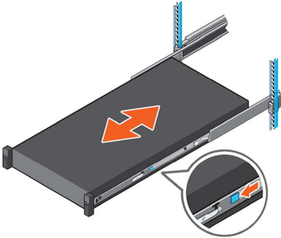
Figure 20. Slide system into the rack
