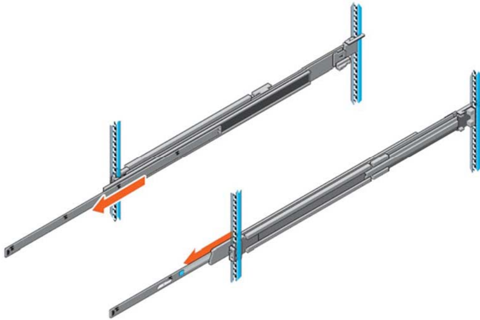
Figure 18. Pull out inner rail
