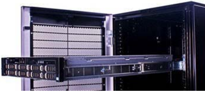
Figure 17. Sliding rails with CMA
