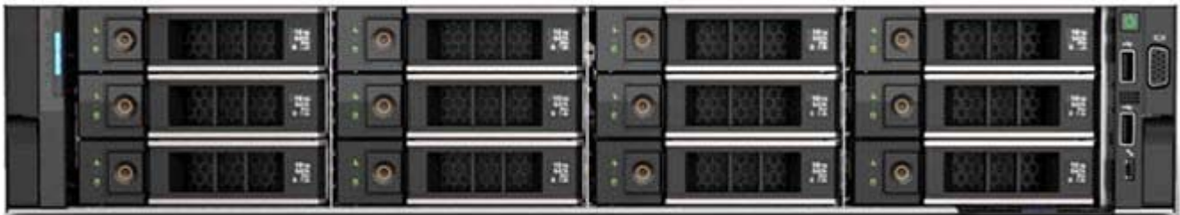
R740xd Front view - 24 x 2.5" hard drive configuration
