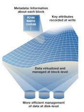
Storage Center to move the blocks to a faster tier of storage. Metadata describing inactive blocks can be used by Storage Center to automatically place the blocks on lower cost, lower performance drives.
