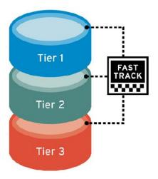
Dell Compellent Fast Track technology enhances Automated Tiered Storage by dynamically placing the most frequently accessed data on the fastest, or outer, tracks of each disk drive. Meanwhile, the least active blocks of data remain on the inner tracks of all the drives in each storage tier. The result is ready access to frequently used data with fewer drives than conventional storage systems.
