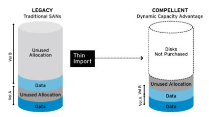
allocated yet unused, and only available to specific applications. Dell Compellent's Thin Provisioning, called Dynamic Capacity, delivers the highest storage utilization possible by eliminating allocated but unused capacity. Dynamic Capacity completely separates storage allocation from utilization, enabling users to create any size virtual volume upfront, yet only consume actual physical capacity when data is written by the application.
