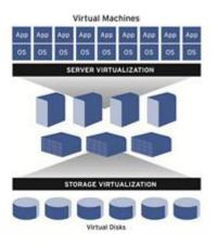
storage pool without disruptions. Virtualization also allows Storage Center to change RAID levels on the fly.
