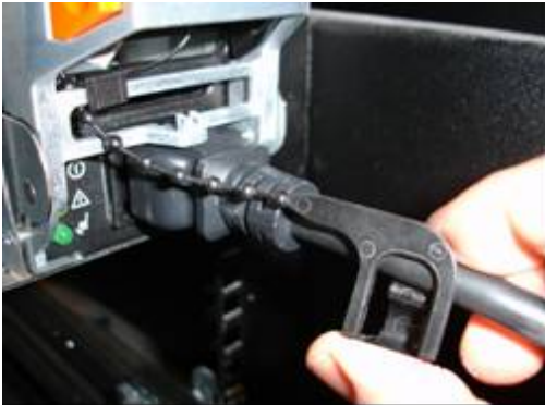
Figure 9c - Clip retainer onto cord
