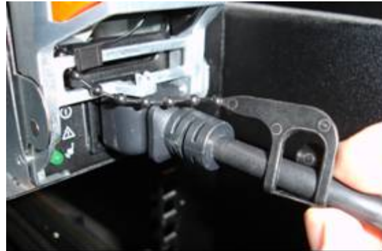
Figure 9d – Retainer clipped onto cord
