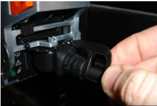
Figure 9e - Slide retainer against overmold
