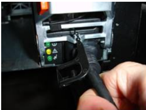
Figure 10c - Remove power cord from PSU
