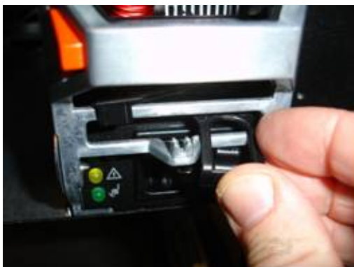
Figure 10e - Re-secure retainer to PSU handle
