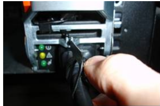
Figure 10b - Flip off retainer with thumb
