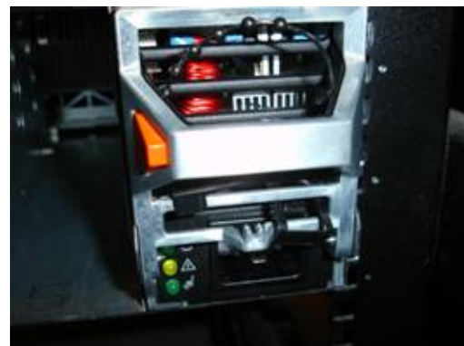
Figure 10f - Retainer secured
