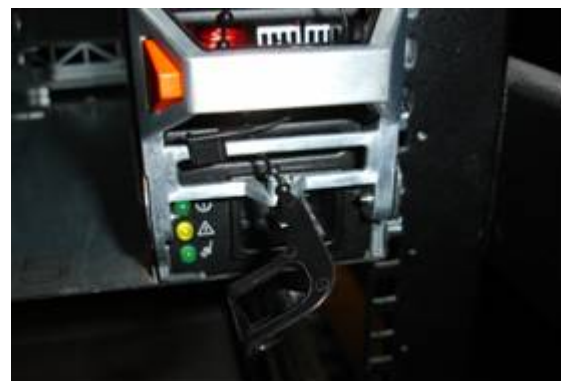
Figure 10d - Power cord removed
