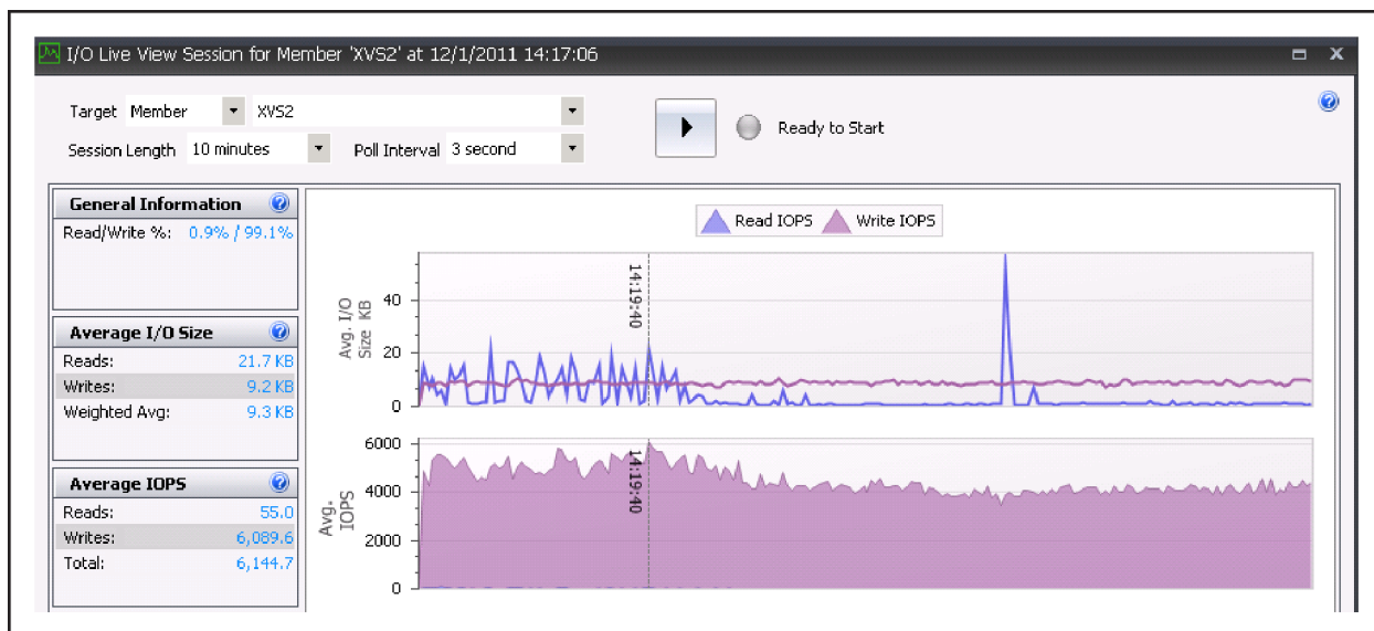
Figure 13 IOPS on one of the EqualLogic array during login storm – 1270 VMs
