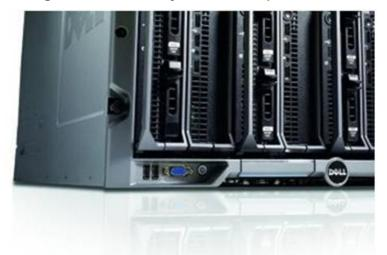
Figure 37. Front keyboard/video ports
