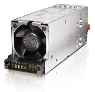
Dell power supplies use output ORing FETs to isolate the power supply from the 12V system bus. If a single power supply fails its output ORing FET, the power supply will turn off removing itself from the bus like an electrical switch that turns off when the power supply fails.
