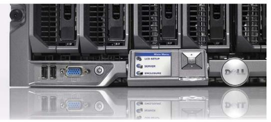
The LCD panel can be used as a diagnostic source and as a place to configure parameters of certain chassis components as well as the server's iDRAC with Lifecycle Controller network configuration. The primary function of the LCD panel is to provide real-time information on the health and status of the modules in the enclosure. LCD panel features include:
