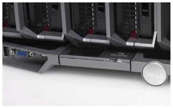
Figure 3. M1000e LCD panel in recessed position
