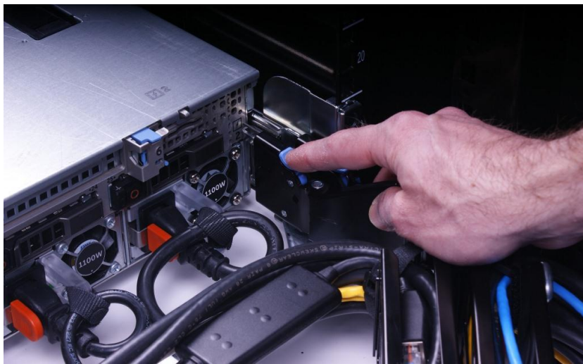
Figure 7. Disconnecting the CMA attachment housings
