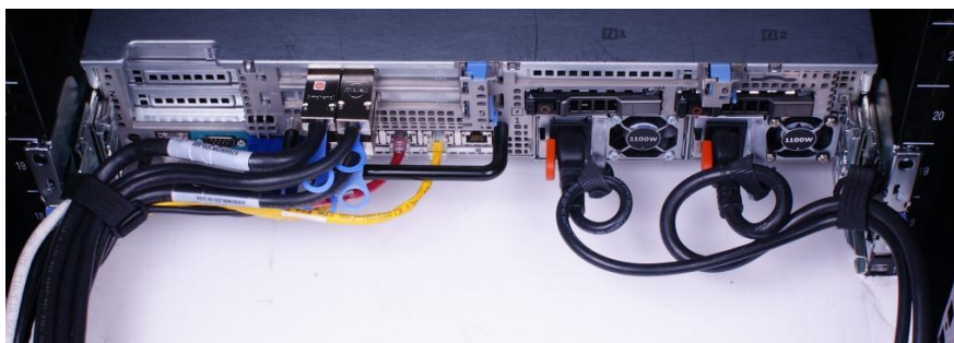
Figure 9. Cable routing without a CMA
