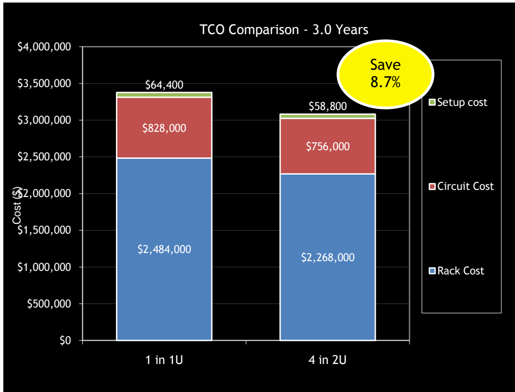
Figure 5: Co-located Data Center TCO Model – Only 3kW Circuit
