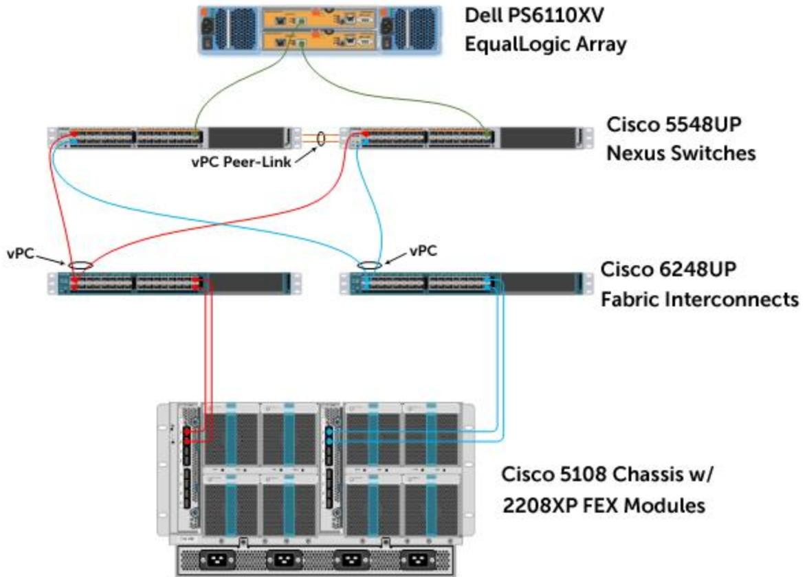
Figure 2. Cisco UCS solution rear view
