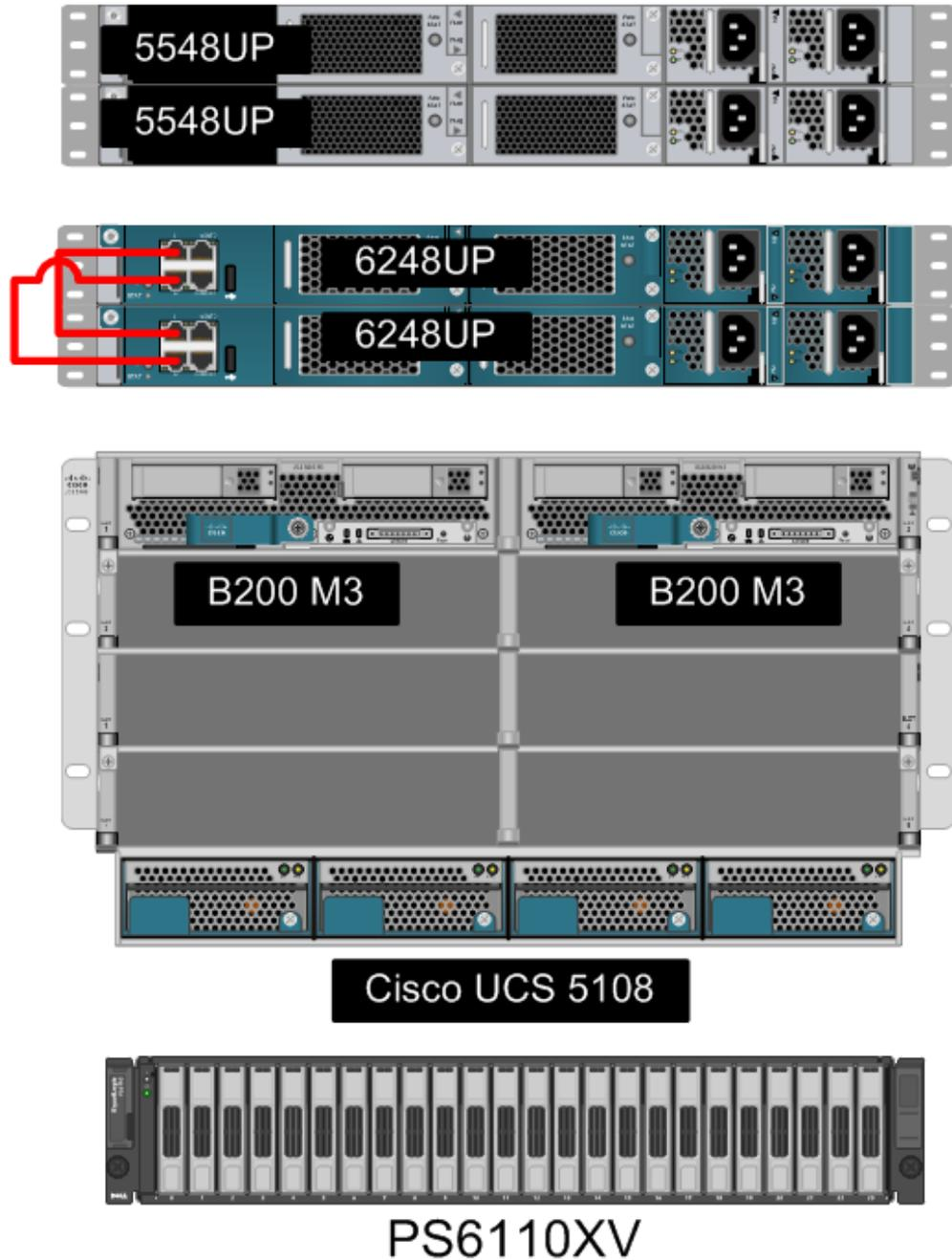
Figure 1. Cisco UCS solution front view
