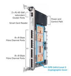
**Figure 12.** Brocade FS8-18 Encryption Blade
