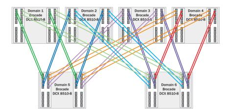
**Figure 7.** Six chassis core-edge topology
