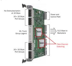
The FC16-48 blade has a higher backplane oversubscription ratio at 16 Gbps but it has larger port groups to take advantage of local switching. Although the backplane connectivity of this blade is identical to the FC16-32 blade, the FC16-48 blade exposes 24 user-facing ports per ASIC rather than 16. Oversubscription occurs only when the first 32 ports are fully utilized. Figure 10 shows a photograph and functional diagram of the FC16-48 blade.
