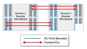
ICLs enable scalable core-edge and active-active mesh chassis topologies. Up to six chassis are supported in a core-edge configuration (see figure 7). This topology will support up to 2304 16 Gbps ports and provide up to 50 Tbps total bandwidth.
