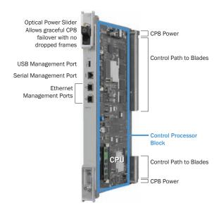
**Figure 2.** CP8 Core Processor Blade
