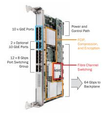
**Figure 13.** Brocade FX8-24 Extension Blade
