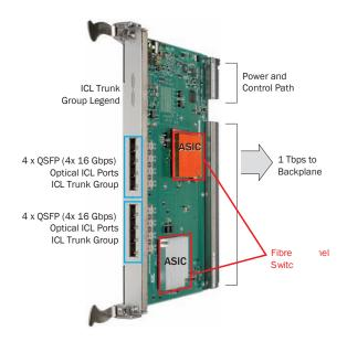
**Figure 4.** CR16-4 Core Routing Blade
