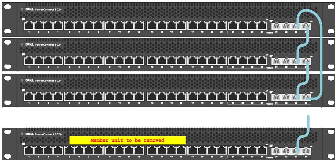
Figure 16. Removal of a stack unit
