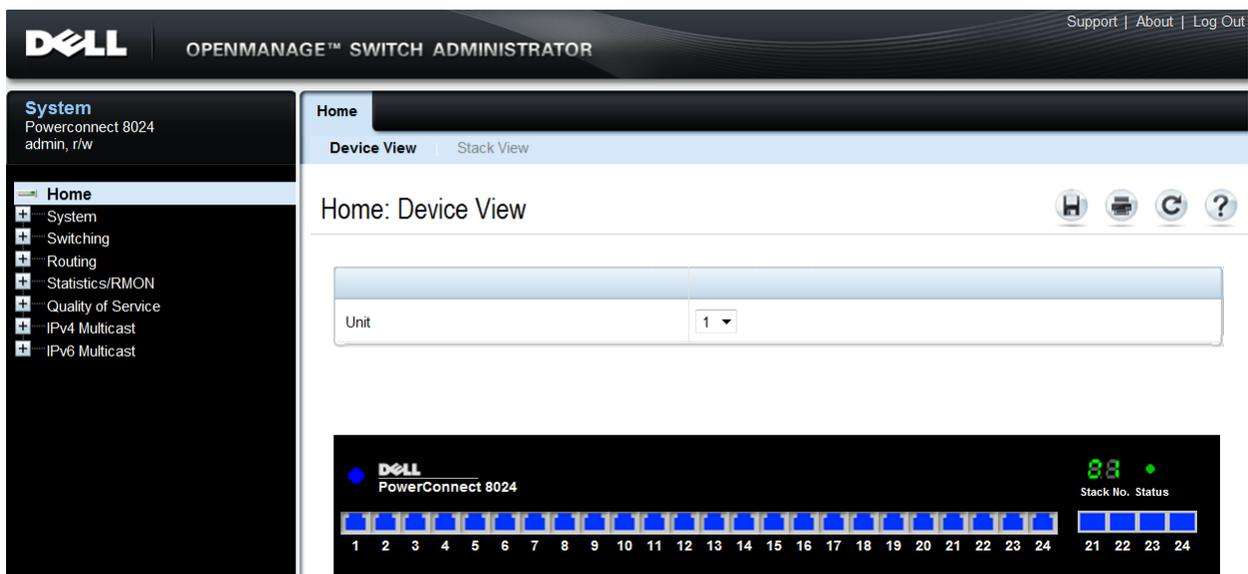
2. Click **System > Stack Management > Stack Port Summary** to bring up the next page used to select the ports for stacking. For this example ports 21 and 22 are used.
