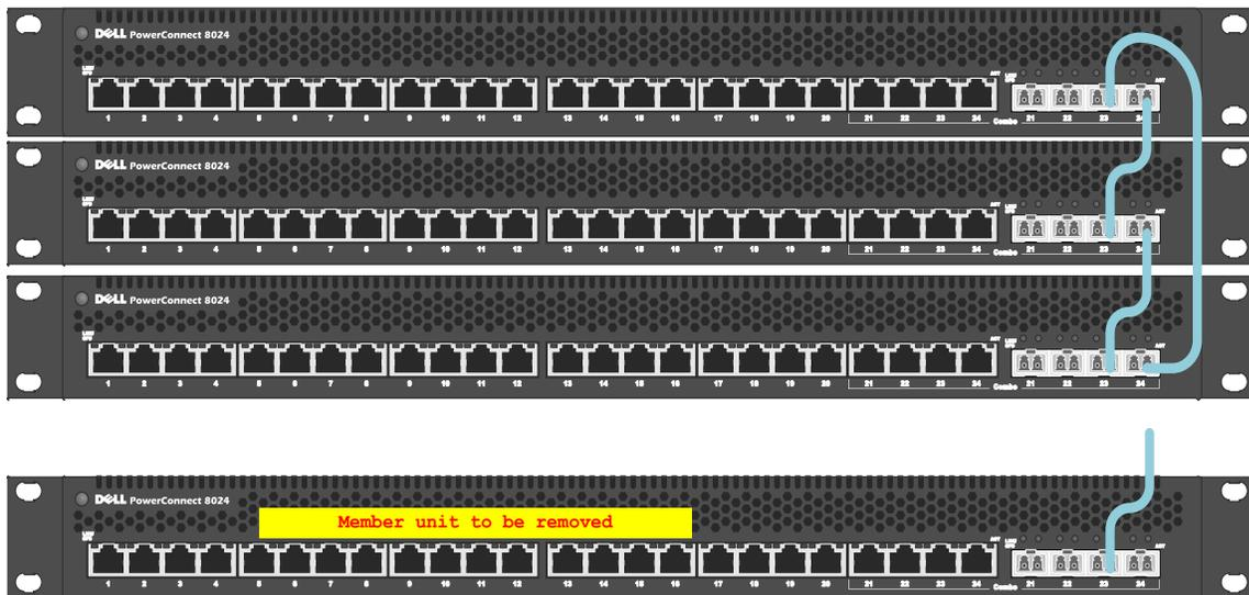
Figure 18. Removal of a stack unit
