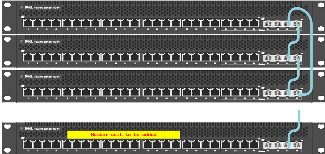
Figure 11. Preparing a Stack Unit (CLI method)
