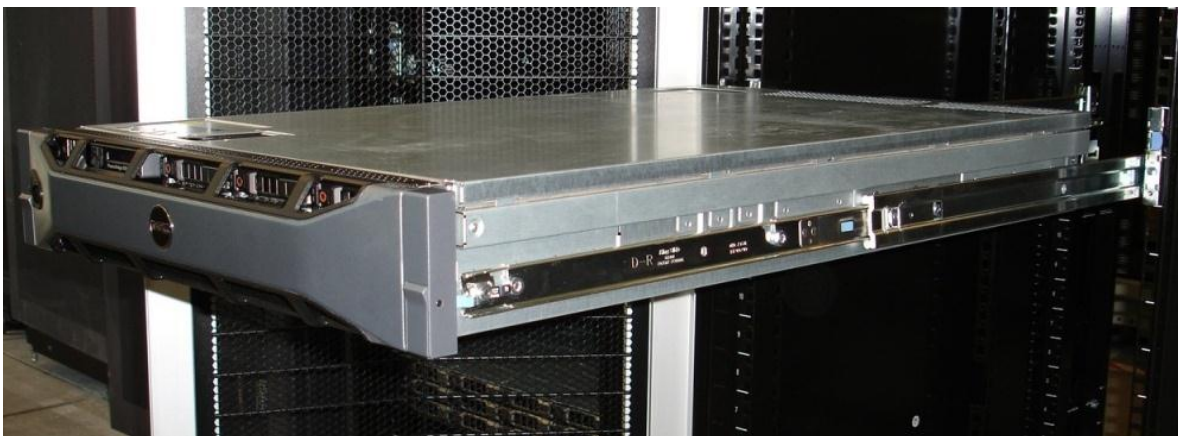
Figure 12. R715 Mounted in the B2 Sliding Rails
