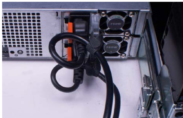
Figure 3. Routing the power cable through the strain relief on a fixed power supply
