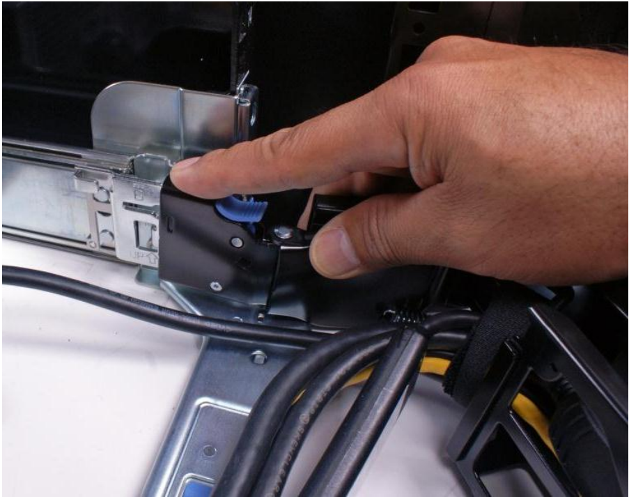
Figure 8. Disconnecting the CMA attachment housings
