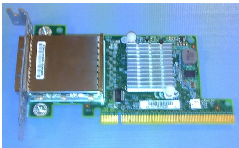
Figure 3. PCIe HIC with external iPASS connector
