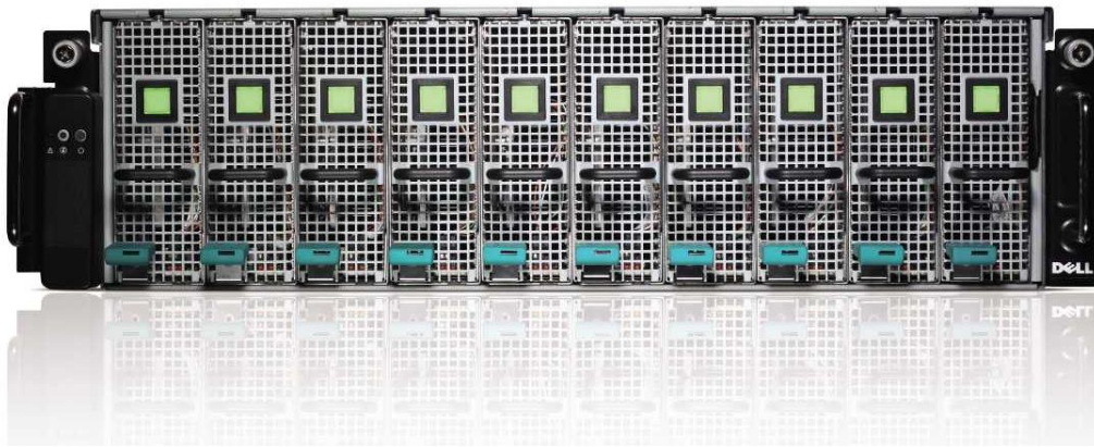
Figure 1. Front panel: C410x expansion chassis
