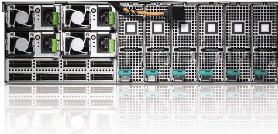
Figure 2. Back panel: C410x expansion chassis
