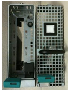
Figure 6. Common carrier and carrier sled module power button LED
