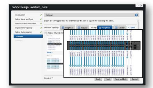
The Fabric Design wizard takes basic input from the user to recommend a series of topology templates, as well as a comprehensive wiring diagram to minimize cabling errors
